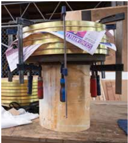
2 Multiple brass table-tops are clamped together for gluing.
