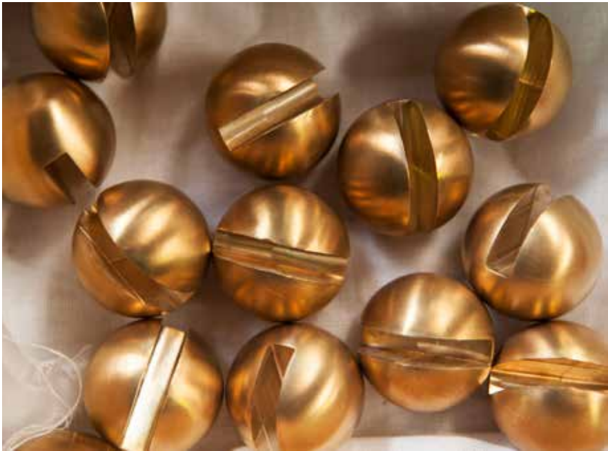
3 Brass spheres with deep grooves slot onto the ends of the table legs to become glides.
